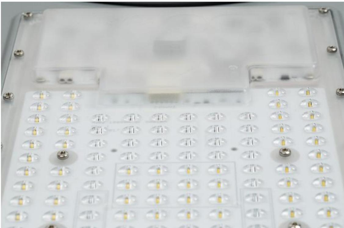
**We have eliminated the need for a driver in the fitting by; a) employing a particular LED system configuration, and b) innovative control circuitry incorporated onto the LED module. It is this advanced electronics engineering that carefully regulates LED current directly from mains voltage.**
