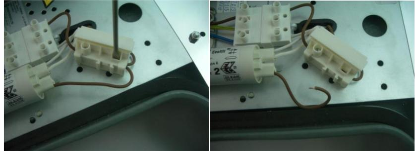
Remove the wire in the capacitor by inserting a small flat blade screwdriver and pull on the wire to release.
